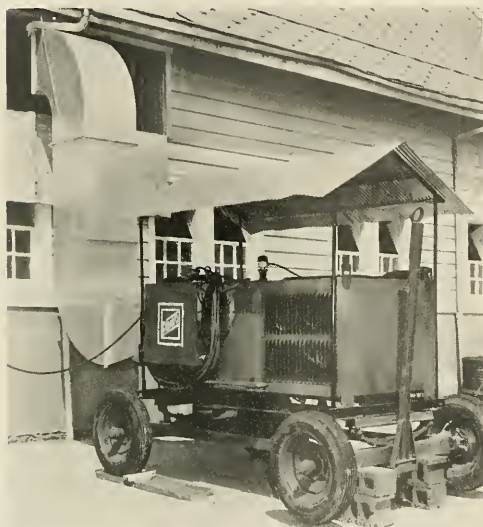
PORTABLE HEATING UNIT is used with new batch type drier; produces enough heat to cause 20° rise in temperature.
